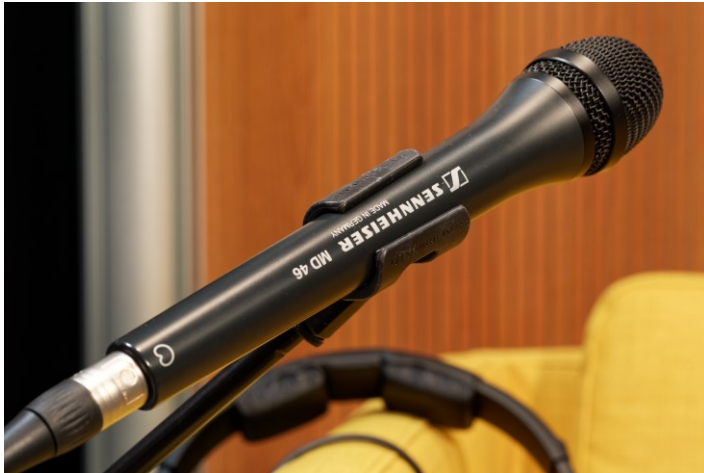
For the podcasts, the speakers' voices are recorded using dynamic Sennheiser MD 46 microphones
